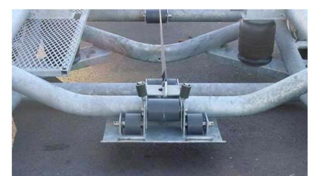
Bird Trailer - The Skid - This will roll on hard surfaces or skid on sand and shingle as used when picking up or droppng the boat from dry land or shore
