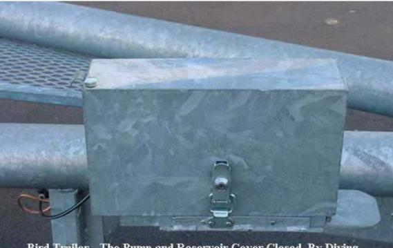
Bird Trailer - The Pump and Reservoir Cover Closed. By Diving Bell principle keeps the Pump and Reservoir in an Air Pocket in the event of Total Immersion, Provides a step into the bows
