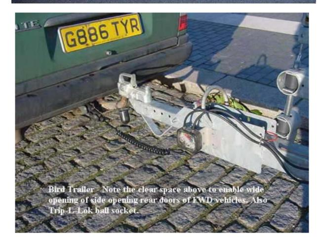
Bird Trailer - The Screwless Jockey Wheel -Also the singlebolt attachment allows rotation in the event of driving off with it down
